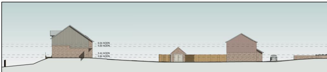
Fig. 4 – Proposed side elevation and site section (1/2 Willop Close to right, proposed house to left)
